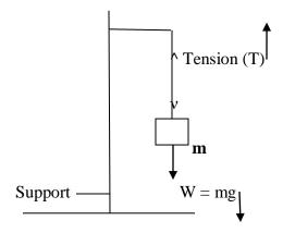
The mass, **m** is suspended on a support using an inextensible string. The force of gravity acts on the mass downwards. The tension force results in the string since it is tied to a rigid support. Two forces act on the mass. i.e. its weight,  $\mathbf{W} = \mathbf{mg}$  and the tension force, **T** (in the string). When the mass is at rest, its acceleration  $\mathbf{a} = \mathbf{0} \ \mathbf{ms}^{-2}$ .
