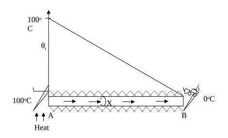
The difference between the temperature distributions is due to the fact that, when the bar is not lagged, heat escapes through its sides by convection. Thus, the heat flowing per second past a
