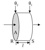
Consider a parallel-sided slab of material of thickness *l*, and area A, with face R at temperature  $\theta_2$  and face S at temperature  $\theta_1$ , where  $\theta_2 > \theta_1$ . The temperature gradient across the slab is  $\frac{\theta_2 - \theta_1}{l}$
