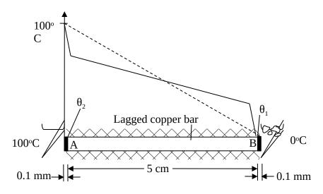
End A of the bar is not at 100°C, and neither is end B at 0°C. To see this, suppose that the conductivity of the dirt is a thousandth that of copper. Then the heat flow rate per second is
