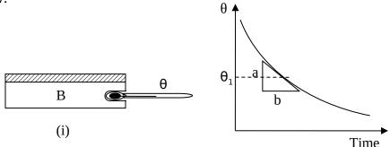
B is now losing heat under the same conditions as in the first part of the experiment. Thus, by drawing a tangent at  $\theta_1$  as shown, the rate of heat loss when B was at  $\theta_1$  is calculated.
