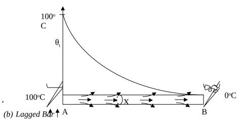
The temperate distribution is uniform along the conductor because no is heat lost to the surrounding.
