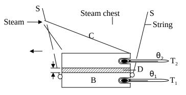
To get an adequate heat flow rate the specimen, D, is made in form of a thin circular disc.
