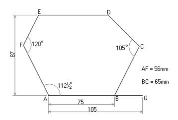
3. Details of a spanner for a hexagonal nut are shown in the figure below. Draw this out line to full size showing clearly all constructions and points of contact.
