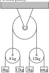
The accelerations of 4kg and 12kg masses are  $\frac{g}{2}$  and  $\frac{g}{2}$  downwards respectively. The accelerations of the 3kg and m kg masses are  $\frac{g}{3}$  upwards and  $\frac{g}{3}$  downwards respectively. The hanging portions of the
