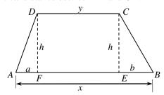
Show that the centre of gravity of the sheet is at a distance  $\frac{h}{3} \left[ \frac{3y+a+b}{x+y} \right]$  from side *AB*.
