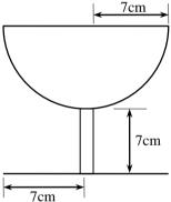
Find the distance from the base, of the centre of gravity of the figure. (Ans: 6.5)
